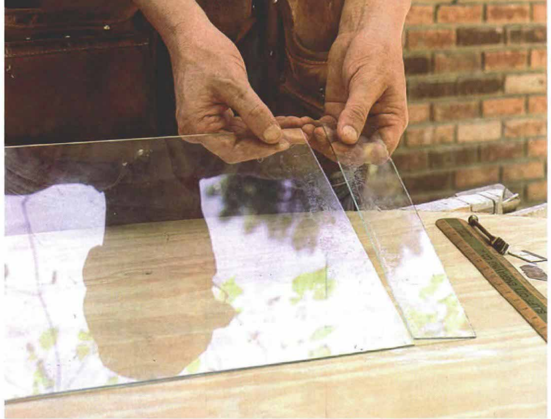
Cutting glass is a snap. After scoring the glass, grip it on both sides of the score mark and apply firm pressure. The pane should break smoothly along the score.
