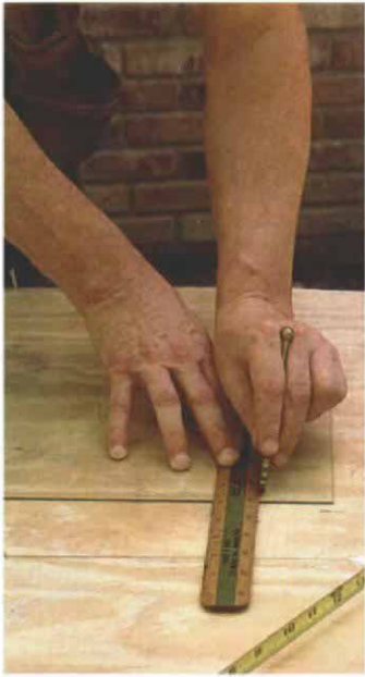
A good cut starts with the right grip. Holding the glass cutter properly is the first key to successful cutting. Apply even pressure and draw the cutter back with a single smooth, continuous motion.
